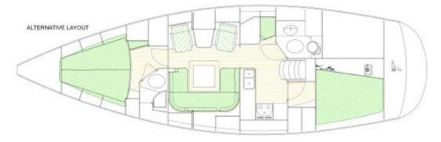
NB! The forward cabin of Malö 40-129 has a v-berth allowing easy access to both berth and the navigation area do not have a seat (this space is used fo more storage and a drawer fridge).
